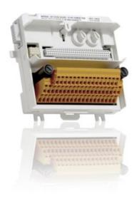
The TU833 MTU can have up to 16 I/O channels and two process voltage connections. Each channel has two I/O connections and one ZP connection. The process voltage can be connected to two individually isolated groups. Each group has a 6.3 A fuse. The maximum rated voltage is 50 V and maximum rated current is 2 A per channel. It is recommended that the fuse rating be chosen to meet the applications needs, see S800 I/O Getting Started chapter Power and Cooling.
