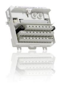
The TU839 MTU can have up to 8 I/O channels and two groups of connections for sensor power distribution. Each channel has two I/O connections. The process voltage can be connected to two individually isolated groups for sensor power distribution. Each group has a 200 mA fuse. The maximum rated voltage is 250 V and maximum rated current is 1 A per channel. It is recommended that the fuse rating be chosen to meet the applications needs.
