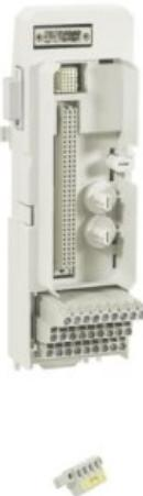
The TU891 MTU has gray terminals for field signals and process voltage connections. The maximum rated voltage is 50 V and maximum rated current is 2 A per channel, but these are primarily constrained to specific values by the design of the I/O modules for their certified application. The MTU distributes the ModuleBus to the I/O module and to the next MTU. It also generates the correct address to the I/O module by shifting the outgoing position signals to the next MTU.
