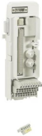
The TU891 MTU has gray terminals for field signals and process voltage connections. The maximum rated voltage is 50 V and maximum rated current is 2 A per channel, but these are primarily constrained to specific values by the design of the I/O modules for their certified application. The MTU distributes the ModuleBus to the I/O module and to the next MTU. It also generates the correct address to the I/O module by shifting the outgoing position signals to the next MTU.
