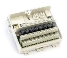
The TU838 MTU can have up to 16 I/O channels. The maximum rated voltage is 50 V and maximum rated current is 3 A per channel. The MTU distributes the ModuleBus to the I/O module and to the next MTU. It also generates the correct address to the I/O module by shifting the outgoing position signals to the next MTU.
