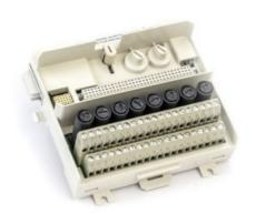
The TU838 MTU can have up to 16 I/O channels. The maximum rated voltage is 50 V and maximum rated current is 3 A per channel. The MTU distributes the ModuleBus to the I/O module and to the next MTU. It also generates the correct address to the I/O module by shifting the outgoing position signals to the next MTU.
