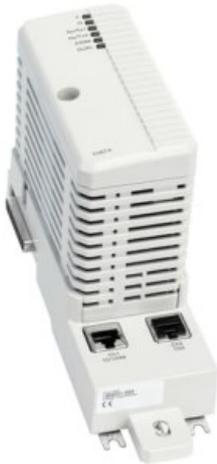
The CI874 is an AC 800M communication interface that connects to external Ethernet devices using the OPC UA protocol. The TP867 Baseplate has one RJ45 Ethernet connector that supports 100Mbps. The CI874 expansion unit contains the CEX-Bus logic, a communication unit, and a DC/DC converter that supplies the required voltage from +24 V supply through the CEX-Bus.
