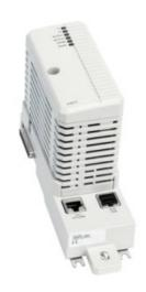
The CI874 is an AC 800M communication interface that connects to external Ethernet devices using the OPC UA protocol. The TP867 Baseplate has one RJ45 Ethernet connector that supports 100Mbps. The CI874 expansion unit contains the CEX-Bus logic, a communication unit, and a DC/DC converter that supplies the required voltage from +24 V supply through the CEX-Bus.
