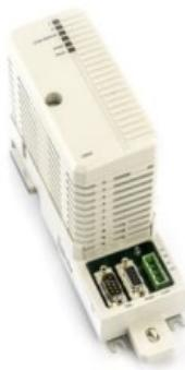
TRIO, interface integrates TRIO/Genius I/O as a native AC 800M I/O. The TRIO interface to the AC 800M is via the CI862 CEX module. This module supports direct connection for one TRIO LAN and provides a port for the Hand Held Monitor.
