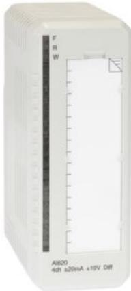
The AI820 Analog Input Module has 4 differential, bipolar current/voltage inputs. Each channel can be either a voltage or current input. The current inputs can withstand an accidental maximum normal mode 30 V d.c. connection. To protect the current input circuit against dangerous input levels, that is, by accidentally connecting a 24 V source, the resistor rating of the 250W current sense resistors is about 5 Watts. This is intended only to temporarily protect one channel at a time.
