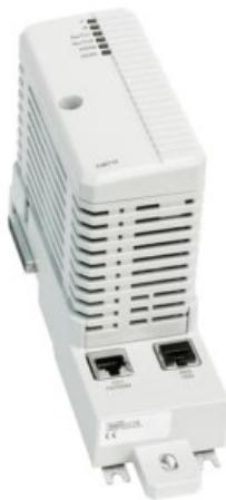
The CI871A is an AC 800M communication interface that connects to the PROFINET IO devices through Ethernet. The TP867 Baseplate has two RJ45 Ethernet connectors, but only the CH1 connector that supports 100Mbps is used for PROFINET IO connection. The Ethernet cable must be connected to the PROFINET IO network through an Ethernet switch.
