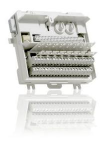
The TU834 MTU can have up to 8 I/O channels and 2+2 process voltage connections. Each channel has two I/O connections and one ZP connection. Input signals are connected via individual shunt sticks, TY801. The maximum rated voltage is 50 V and maximum rated current is 2 A per channel. The MTU distributes the ModuleBus to the next MTU. It also generates the correct address to the I/O modules by shifting the outgoing position signals to the next MTU.
