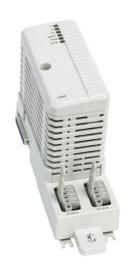
The CI869 is an AC 800M communication interface that connects to the AF 100 field bus through the twisted pair (TWP). The CI869 expansion unit contains the CEX-Bus logic, a communication unit, and a DC/DC converter that supplies the required voltage from +24 V supply through the CEX-Bus. The CI869 can be configured for both redundant cables and redundant communication interfaces.
