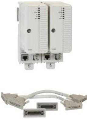
The CEX-Bus unit BC820 is used for extending the onboard communication ports with communication interface units. It is also possible to use redundant communication interfaces on the CEX-Bus. The BC820 CEX-Bus Interconnection Unit offers a way to section the CEX-Bus into two independent segments up to 200 meters apart. This improves availability in systems with redundant communication interfaces.
