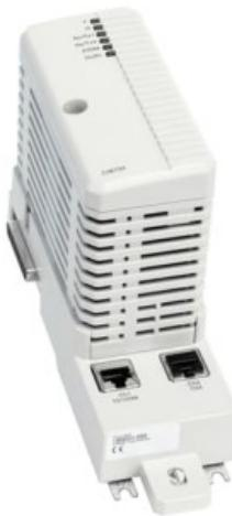
The CI873A is an AC 800M communication interface that connects to external Ethernet devices using the EtherNet/IP protocol. The TP867 Baseplate has two RJ45 Ethernet connectors, but only the CH1 connector that supports 100Mbps is used. The CI873 expansion unit contains the CEX-Bus logic, a communication unit, and a DC/DC converter that supplies the required voltage from +24 V supply through the CEX-Bus.
