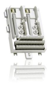
The TU842 MTU can have up to 16 I/O channels and 2+2 process voltage connections. Each channel has two I/O connections and one ZP connection. The maximum rated voltage is 50 V and maximum rated current is 3 A per channel.
