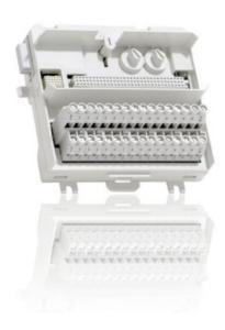
The TU851 MTU can have up to 16 I/O channels. The maximum rated voltage is 250 V and maximum rated current is 3 A per channel. The MTU distributes the ModuleBus to the I/O module and to the next MTU. It also generates the correct address to the I/O module by shifting the outgoing position signals to the next MTU.
