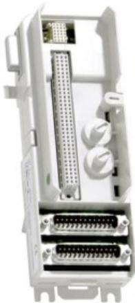
The TU830V1 MTU can have up to 16 I/O channels and two process voltage connections. Each channel has two I/O connections and one ZP connection. The MTU is a passive unit used for connection of the field wiring to the I/O modules. It also contains a part of the ModuleBus.
