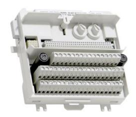
The TU830V1 MTU can have up to 16 I/O channels and two process voltage connections. Each channel has two I/O connections and one ZP connection. The MTU is a passive unit used for connection of the field wiring to the I/O modules. It also contains a part of the ModuleBus.
