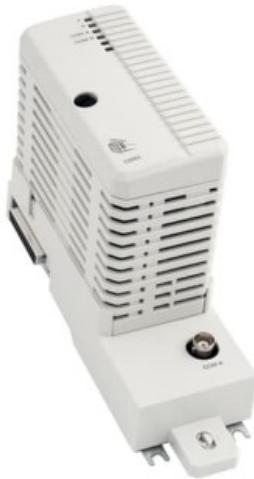
The CI865 module is the AC 800M system's communication interface for Satt ControlNet and bridges different bus standards used on AC 800M and Satt ControlNet. The CI865 module makes it possible to use older Satt I/O system (Rack I/O and Series 200 I/O) with the AC 800M controller platform, but it cannot be used as a general ControlNet interface. CI865 cannot be used in a High Integrity controller.
