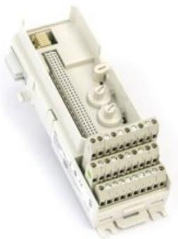
The TU811V1 is a 8 channel 250 V compact module termination unit (MTU) for the S800 I/O. The MTU is a passive unit used for connection of the field wiring to the I/O modules. It also contains a part of the ModuleBus.
