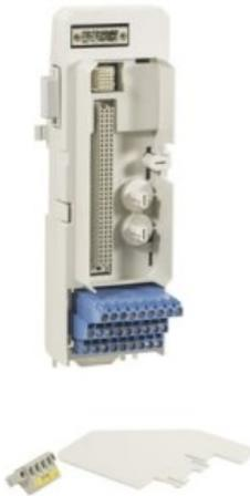
The TU890 is a compact MTU for the S800 I/O. The MTU is a passive unit used for connecting the field wiring and power supply to the I/O modules. It also contains a part of the ModuleBus. The TU890 MTU has gray terminals for field signals and process voltage connections. The maximum rated voltage is 50 V, and the maximum rated current is 2 A per channel, but these are primarily constrained to specific values by the design of the I/O modules for their certified application.
