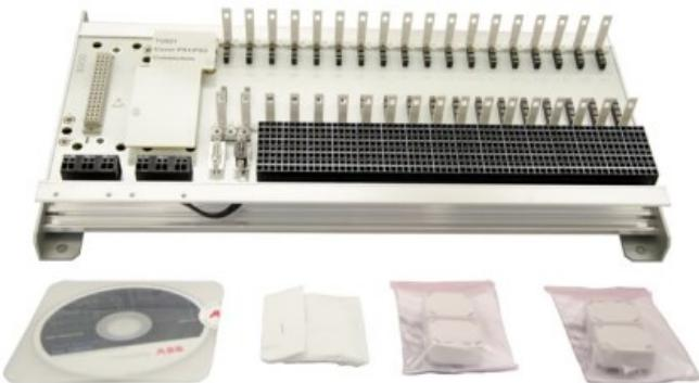
The remote S900 I/O system can be installed in non-hazardous areas or directly in Zone 1 or Zone 2 hazardous area depending on the selected system variant. S900 I/O communicates with the control system level using the PROFIBUS DP standard. The I/O system can be installed directly in the field, therefore the costs for marshalling and wiring are reduced.
