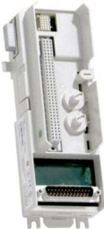
The TU812V1 is a 50 V compact module termination unit (MTU) for the S800 I/O system with 16 signal connections. The MTU is a passive unit used for connection of the field wiring. It also contains a part of the ModuleBus.
