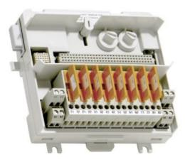
The TU836V1 MTU can have up to 8 I/O channels. The maximum rated voltage is 250 V and maximum rated current is 3 A per channel. The MTU distributes the ModuleBus to the I/O module and to the next MTU. It also generates the correct address to the I/O module by shifting the outgoing position signals to the next MTU.
