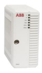
S800 I/O is a comprehensive, distributed and modular process I/O system that communicates with parent controllers and PLCs over industry-standard field buses. The TB840 ModuleBus Modem is a fiber optic interface to the Optical ModuleBus. TB840A is used in redundancy configurations where each module is connected to different optical ModuleBus lines, but connected to the same electrical ModuleBus.
