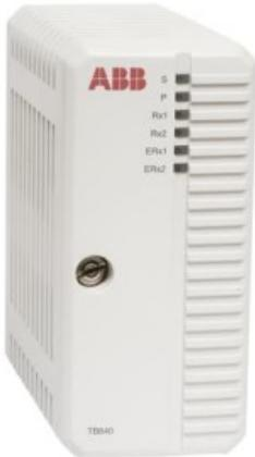
S800 I/O is a comprehensive, distributed and modular process I/O system that communicates with parent controllers and PLCs over industry-standard field buses. The TB840 ModuleBus Modem is a fiber optic interface to the Optical ModuleBus. TB840A is used in redundancy configurations where each module is connected to different optical ModuleBus lines, but connected to the same electrical ModuleBus.
